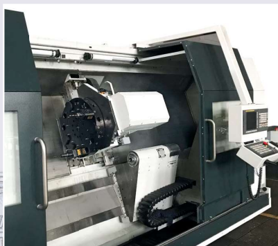
FCT 700 x 1600 with 12 position disc turret with integrated Y-axis
