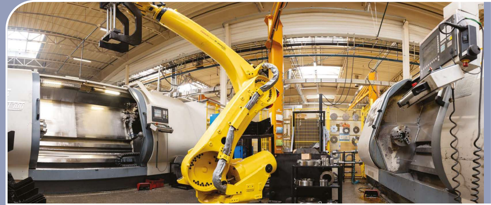
Two FCT700 lathes working with an integrated robot
