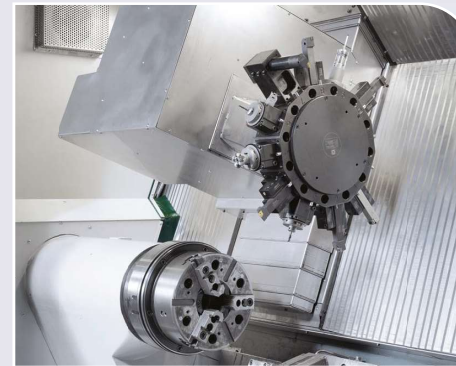
12 position turret radial Tool drive and integrated Y Axis
