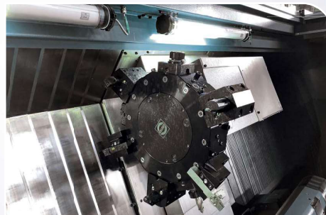
FCT700 - turning length 5.100mm (201"). Automatic door Independent tailstock NC drive and hydraulic steady rest. Turret with driven tools.
