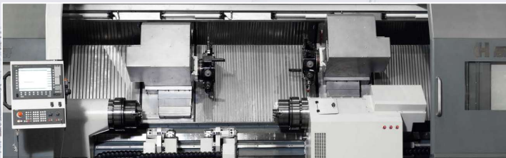
FCT700 with 840 mm (33") increased swing over bed and 2 independent carriages.
