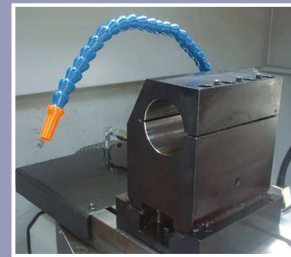
Boring bar attachment mounted on cross-slide T slots
