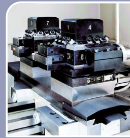
Combination of 2 horizontal head turrets
