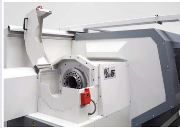
Second spindle nose with complete interlocked covers
