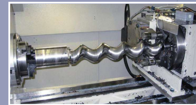
Installation of whirling unit
