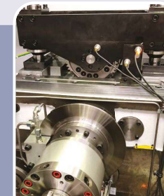
Headstock with full contouring C axis and actuating cylinder for hydraulic chuck
